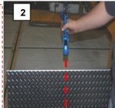
Only lift vertically. Make horizontal adjustments to the position of the clamp by moving the hoist. DO NOT push or pull the clamp so that the hoist chain/rope is not vertical. This is important because any deflection of the chain/rope from straight upand-down will cause the load to swing when lifted. A swinging load may cause serious personal injuries
