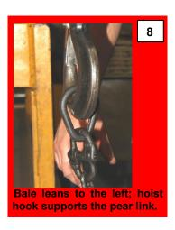
**STEP 8:** Release the load. Rotate the latch lever to the unlocked position. Pull the clamp off of the sheet; then disconnect the clamp from the hoist hook. NOTE: It might be necessary to wiggle the clamp to loosen the connection between the gripper and the sheet.
