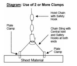
**STEP 6:** Lift the sheet to an ergonomically comfortable height. Steady the load by grasping the hoist hook or the bale of the clamp. Do not apply any weight to the top edge of the sheet material. Do not touch the lock lever. Walk slowly and move the load to the work location.
