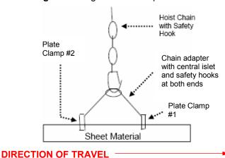
**STEP 7:** Make sure that the load is not swinging or rotating. Slowly lower the hoist hook until the load contacts the ground or work surface. Lower the load sufficiently to create slack in the clamp chain. DO NOT disconnect the clamp from the sheet until the material has been stabilized. **If you cannot control BOTH the clamp and sheet material without difficulty, ask someone to help you**.
